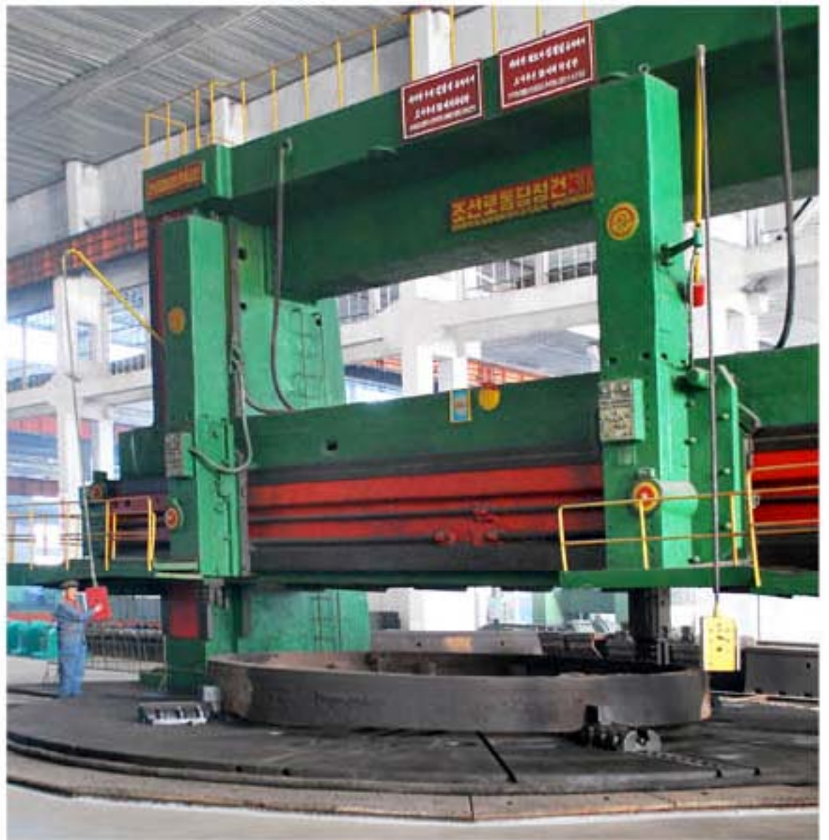
Gear production by means of an 18-metre turning lathe.
