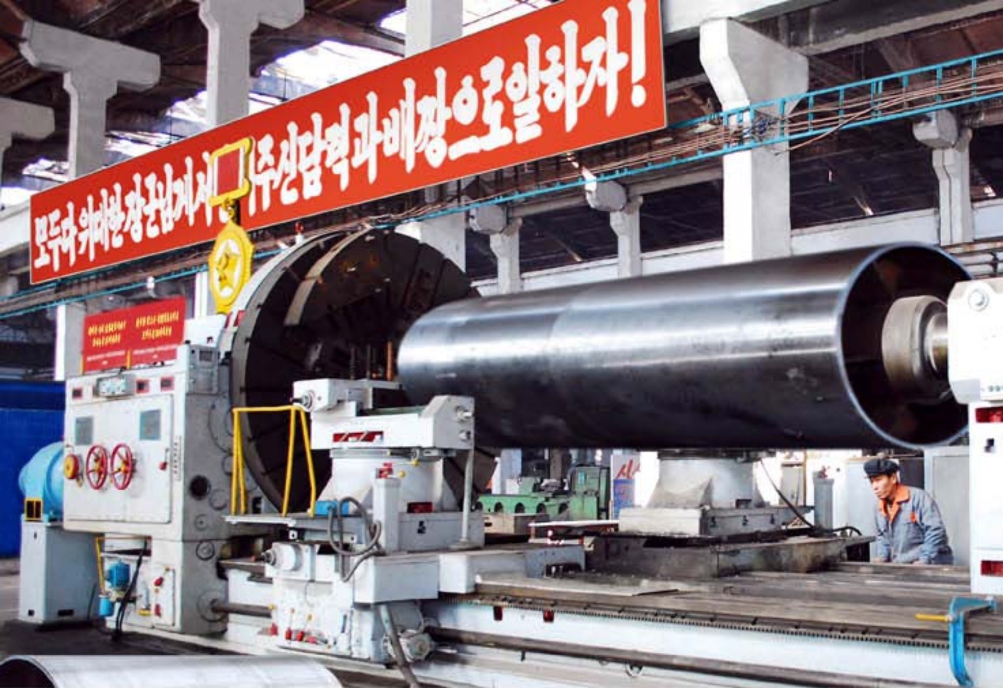
Manufacturing by means of a 20-metre lathe.
